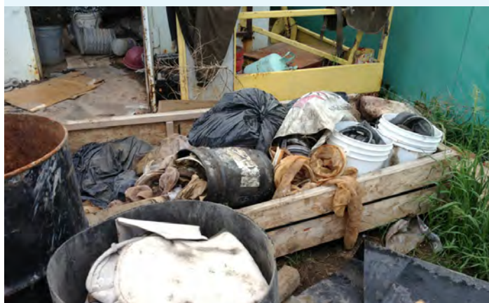
Used filter socks among other debris at a fracking site in North Dakota.
